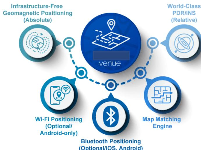
VENUE can accurately present location information even indoors with its unique positioning technology: a combination of geomagnetic sensors, accelerometers, and gyroscopic sensors, as well as Bluetooth and Wi-Fi.
